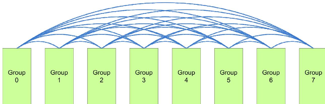
$$\text{bisection bandwidth} = \text{link bandwidth} \times \frac{\text{group optical ports}}{\text{groups} - 1} \times \text{groups}$$
