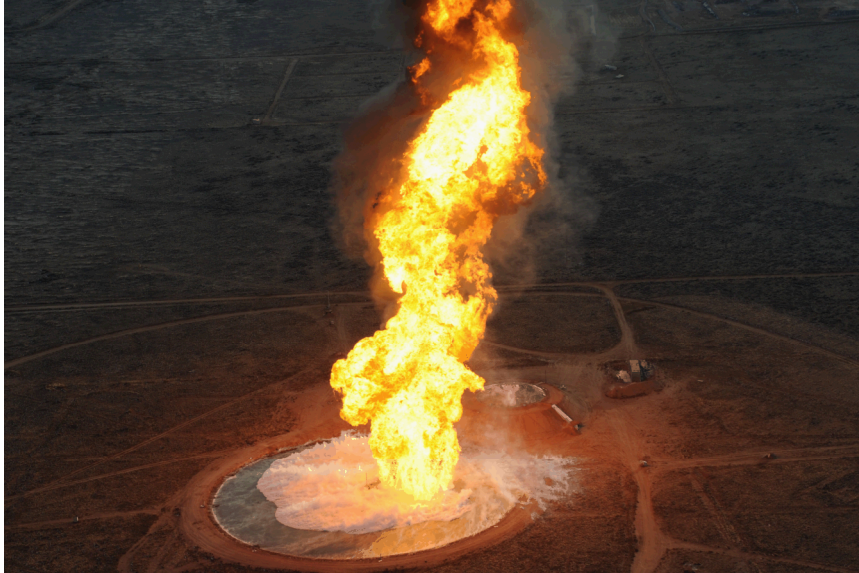
A large scale LNG spreading pool fire on water.
