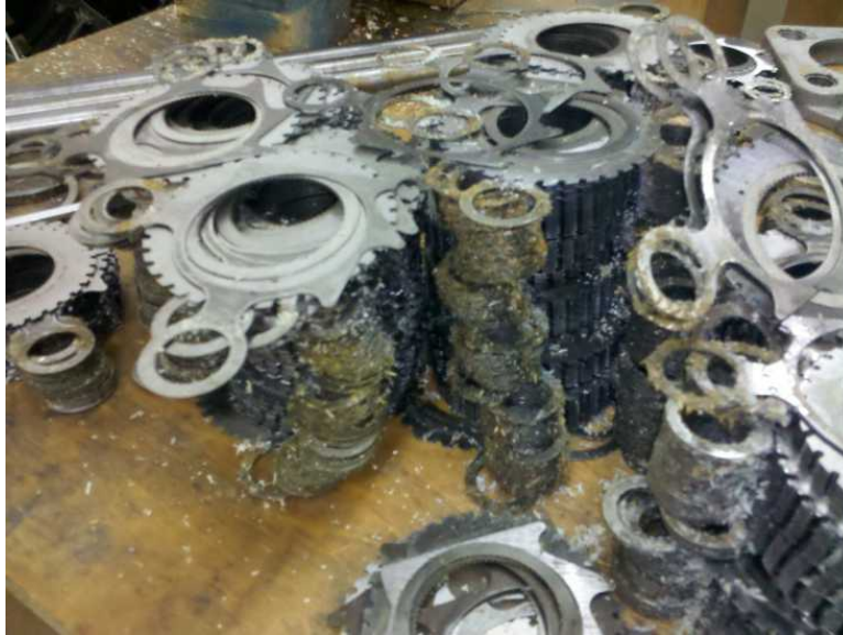
Figure 1: A standard issue of low quality machine oils is gumming-up in shredder blades; particular attention was given to identifying this issue throughout the evaluation.
