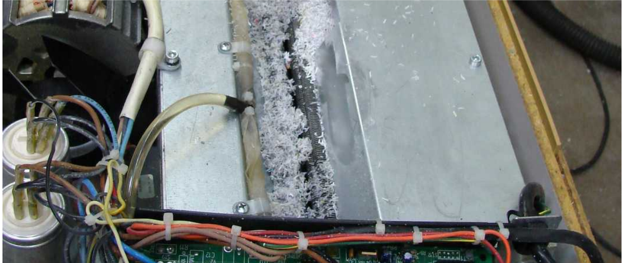
Figure 3: Dahle shredder head, cover, and wick at end of evaluation
