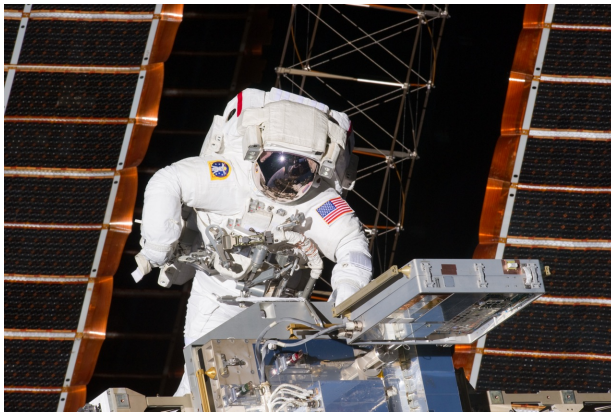
Exterior of the international space station, showing the MISSE experiments being secured by an astronaut.
