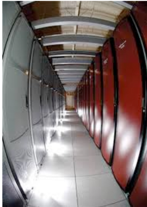
A portion of the cabinetry containing some of the thousands of processor racks comprising Sandia’s Red Storm massively parallel supercomputer.
