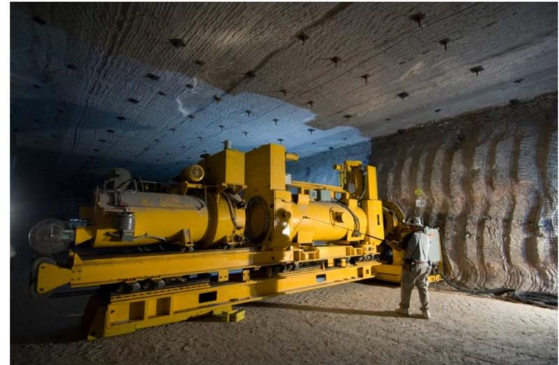
**Emplacement of remote-handled (RM) waste in the wall of a WIPP panel**
