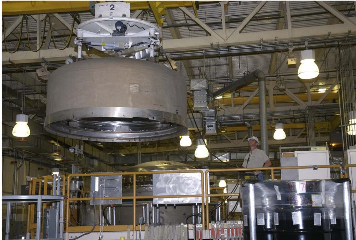
In this picture, the TRUPACT-II is in the WIPP Waste Handling Building TRU-dock to be unloaded. The Outer Containment Vessel (OCV) lid is being removed and will be placed on the round (grey) rack in the lower left corner of the picture. After the OCV lid is removed, the ICV will be removed in a similar fashion, allowing access to the waste packages within the ICV. The Inner Containment Vessel (ICV) lid can be seen as it remains on the TRUPACT-II container.
