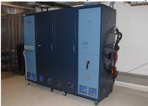
72 V 1000 A Bitrode (2 Parallel Channels)
