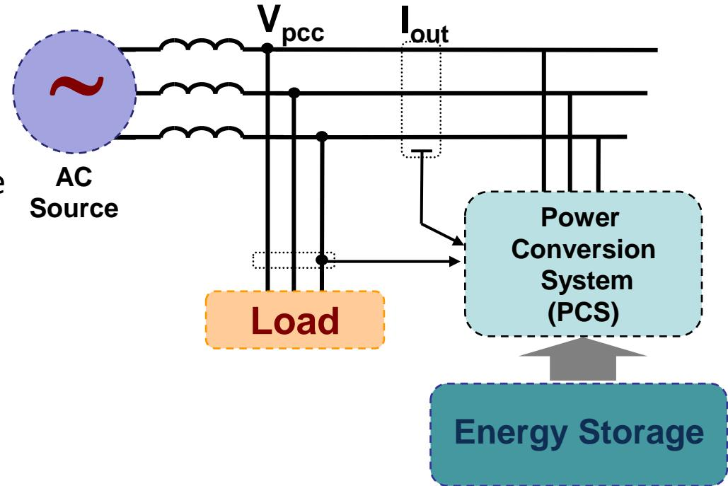
*The PCS is a key component of the energy storage system—it can represent 20-60% of the total system cost.*
