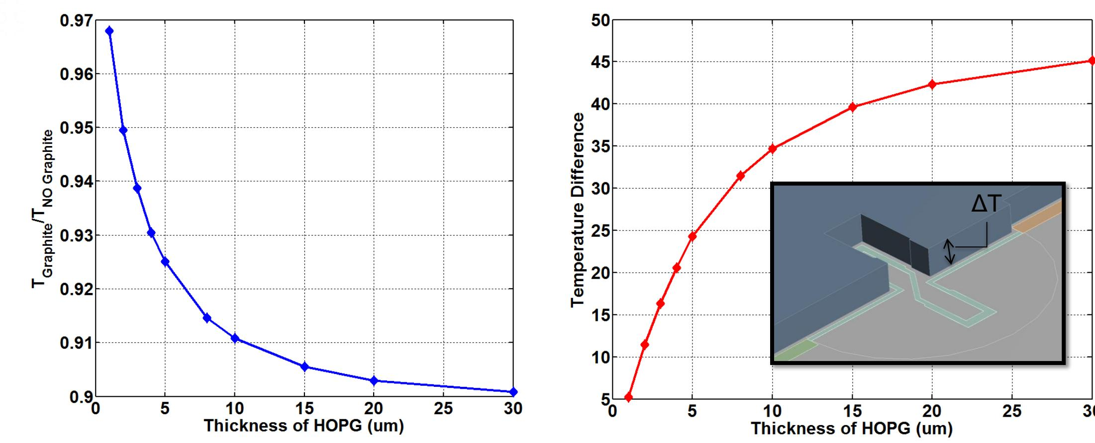
Low cross plane thermal conductivity limits usefulness of increasing graphite thickness.
