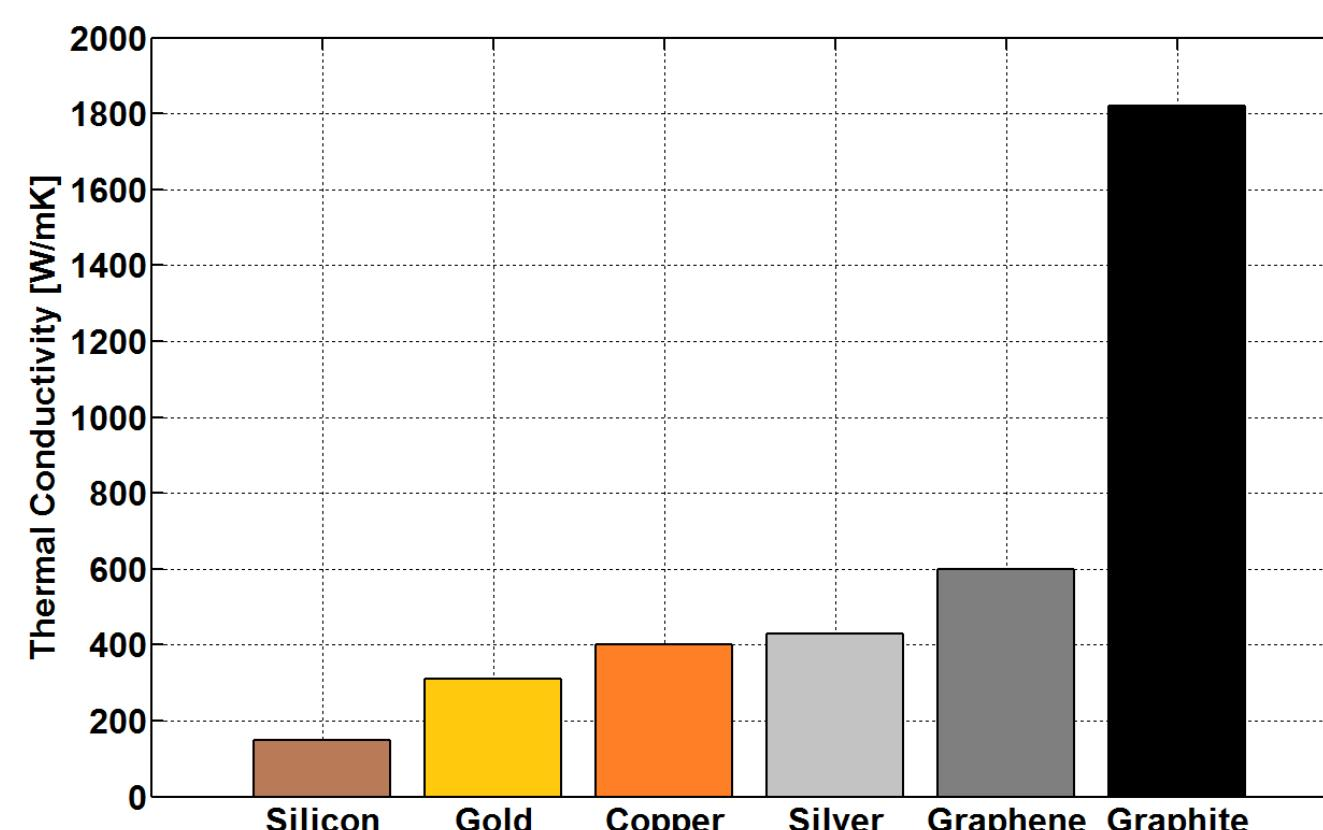
Graphene(ite) materials have extremely high thermal conductivities
