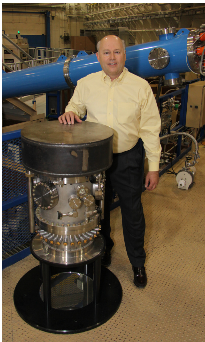
Randy with the plutonium containment system used on the Z machine.
