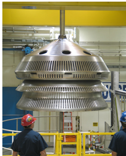
Lower three MITLs suspended under Z facility 40,000 pound crane
