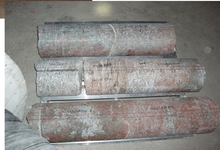
300 mm Diameter WIPP Core.
