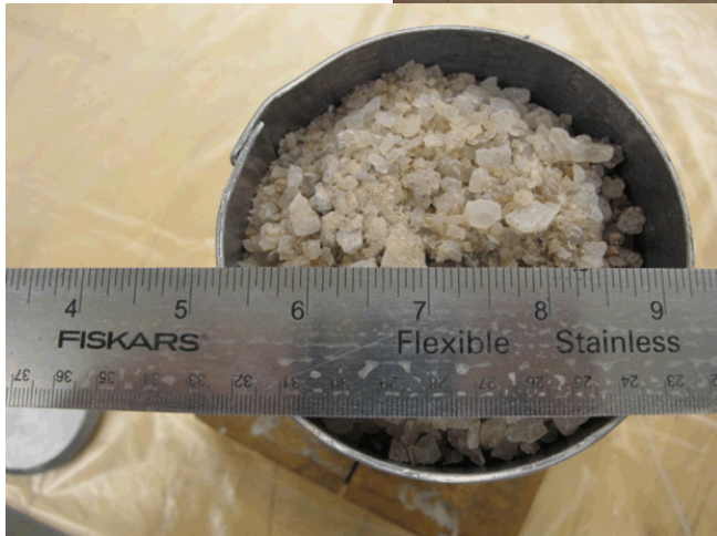
Sieved Run-of-Mine WIPP Salt used in Testing.
