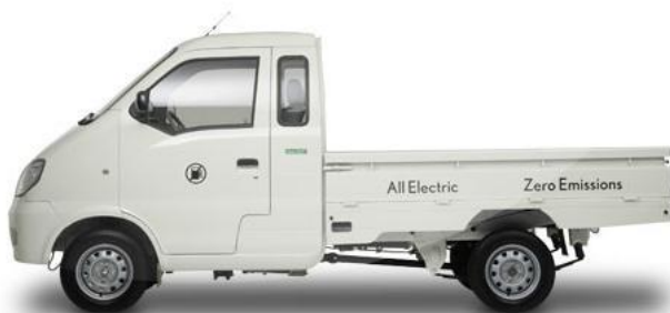
Figure 1. Miles Electric model ZX40ST battery electric work truck used by the City of Santa Monica.
