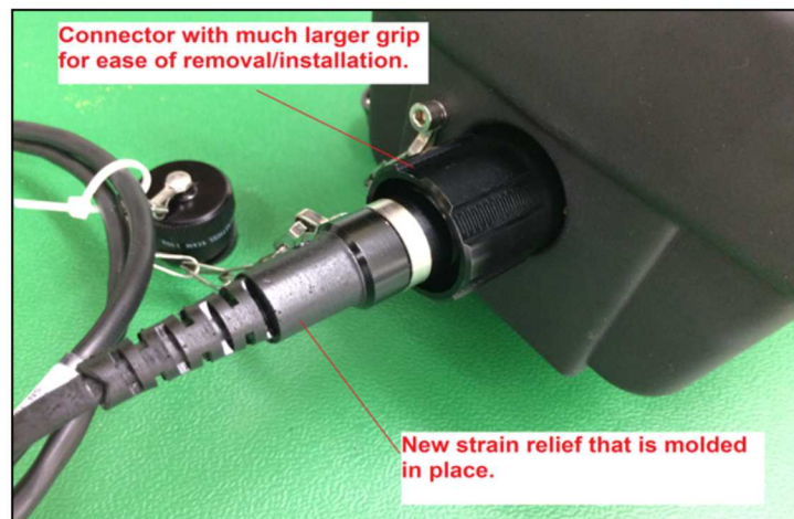
New Strain Relief and Connector Backshell
