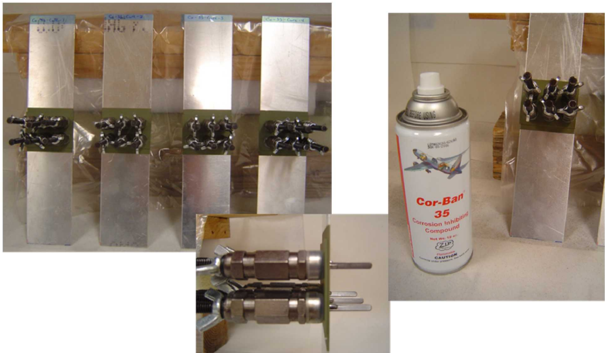
Figure 5-28: CIC Cure Assessment Coupons with Clecos at Rivet Points
