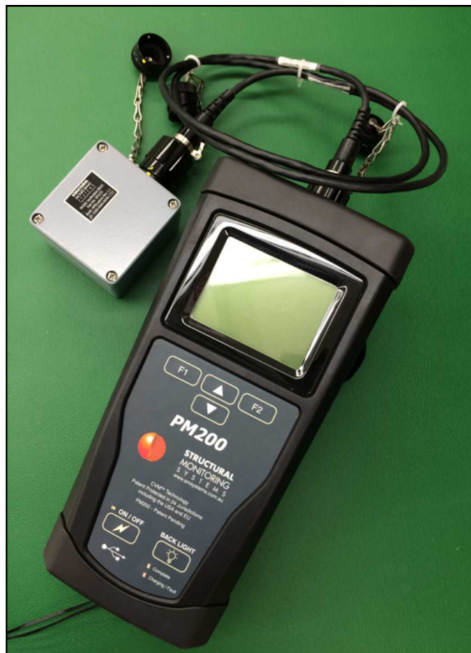
Figure 8-7: Verification Block for In-Situ Calibration of PM200 Instrument
