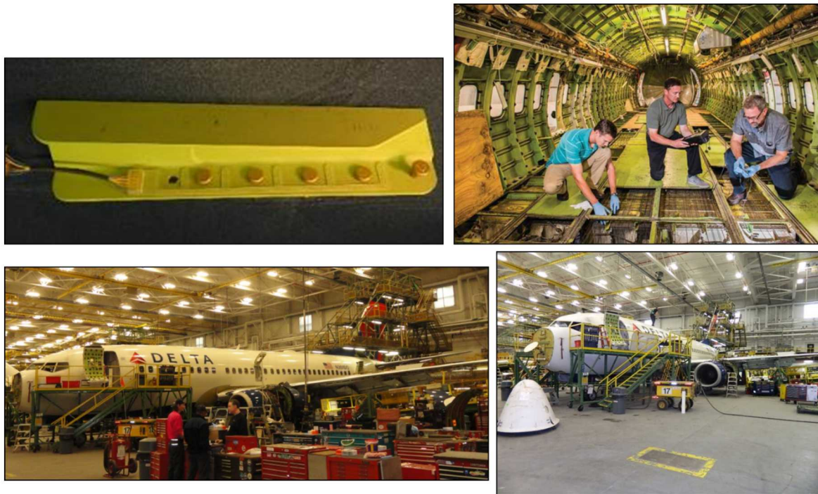
Figure 6-8: Overview of CVM Sensor Installations on Wing Box Fittings at Delta Facility
