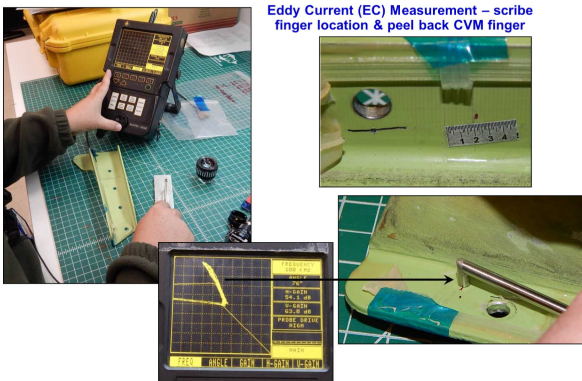
Figure 4-13: Crack Length Measured with Eddy Current Inspections to Plot Data with Associated dCVM Levels Measured by PM-200
