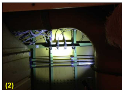
Removal of Baggage Liner to Access 4 SLS Connectors Mounted to Bulkhead
