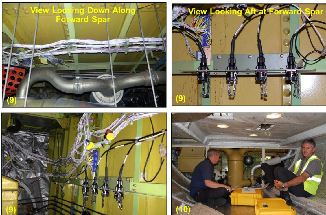
Figure 6-18: CVM Installation and Monitoring - 9) Connection of Multiple CVM Sensors to Individual SLS Connectors and 10) Monitoring CVM with PM-200 Device
