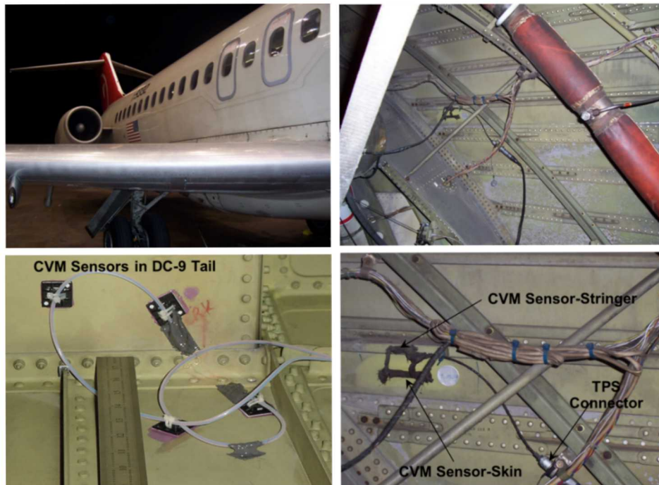
Figure 6-2: Sample CVM Installations on Aircraft in the Northwest Airlines Fleet
