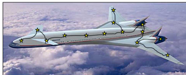
Figure 1-1: Depiction of Distributed Network of Sensors to Monitor Structural Health
