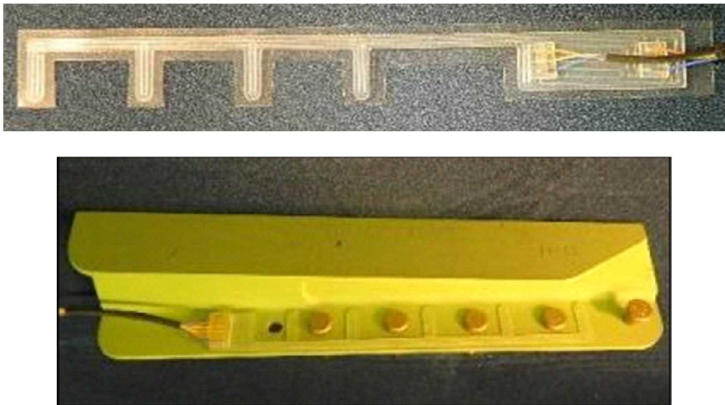
Figure 3-7: CVM Sensor Mounted on Wing Box Fitting to Monitor All Inspection Regions
