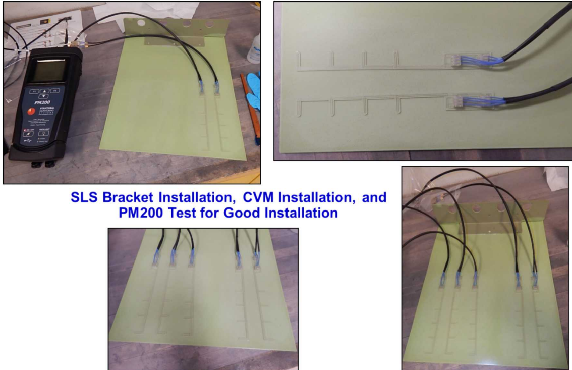
Figure 5-7: Installation of Five Wing Box CVM Sensors for Environmental Durability Test
