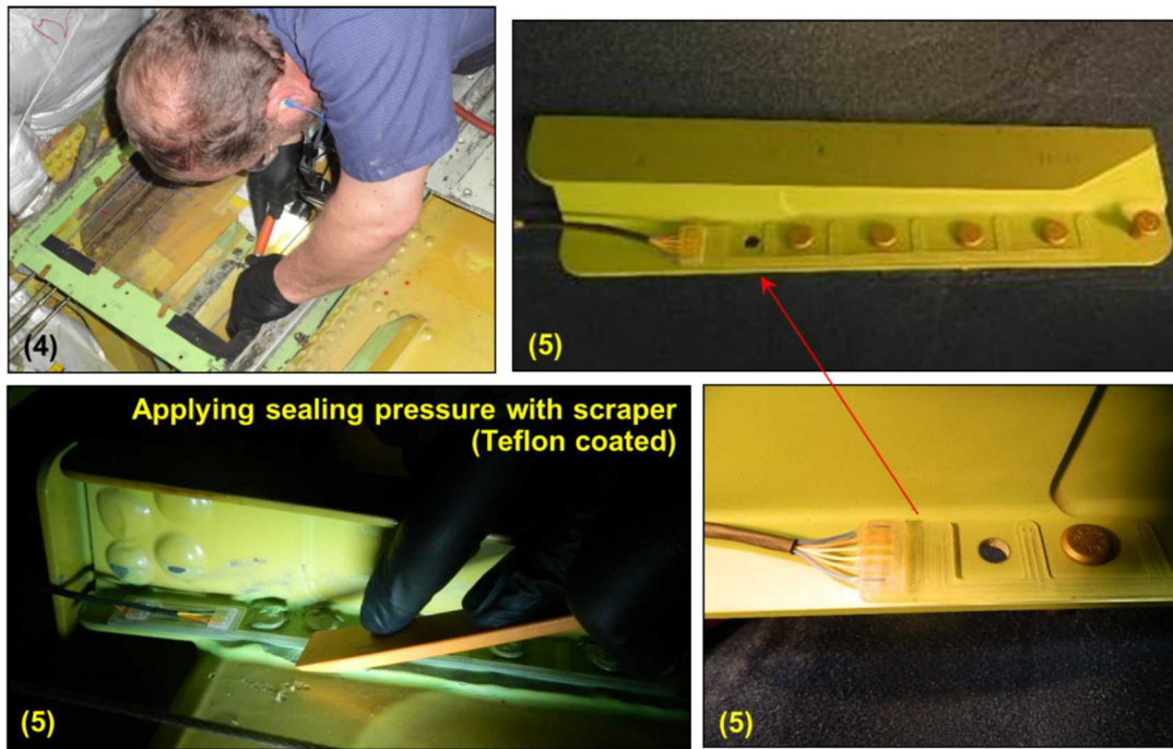
Figure 6-16: CVM Installation Steps - 4) CVM Surface Preparation (light sanding, acetone & deionized water clean), and 5) CVM Sensor Placement on Wing Box Fitting
