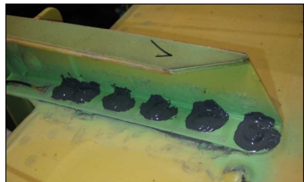
Installed Sensor, prior to FVB overcoat
