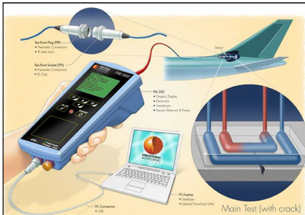
Figure 2-9: Comparative Vacuum Monitoring System
