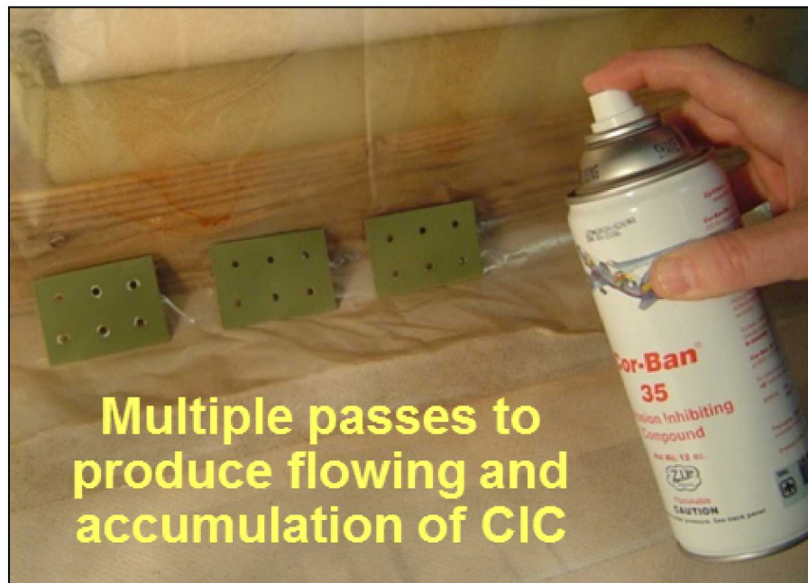
Figure 5-29: Application of BMS 3-35 (Corban-35) Corrosion Inhibiting Compound to Evaluate Cure Time and Flow of CIC Compounds
