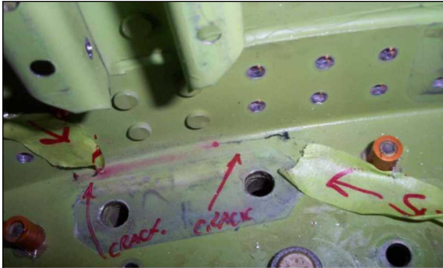
Figure 7-26: Possible SHM Application – Cracks in Bulkhead Outer Chord
