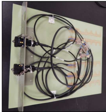
Figure 5-9: Final Sensor Set-Up into Groupings as those used on Operational Aircraft
