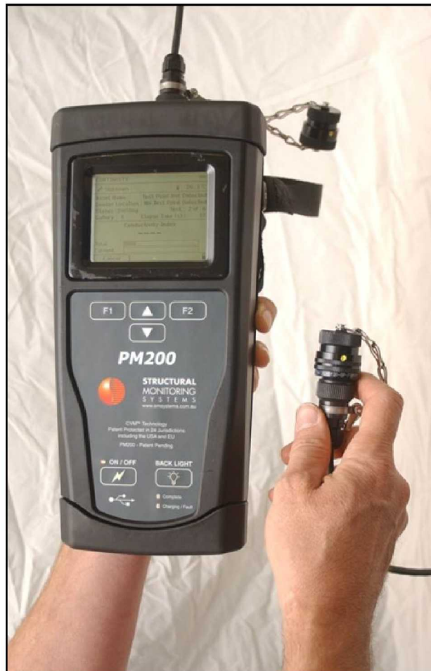
Figure 8-6: PM200 Device Used to Interrogate CVM Sensors and Perform Structural Monitoring
