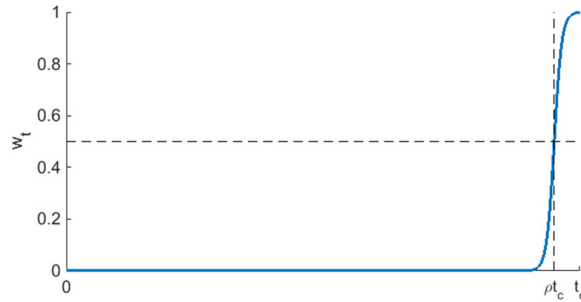
Figure 4.19 Soft constraint for travel time
