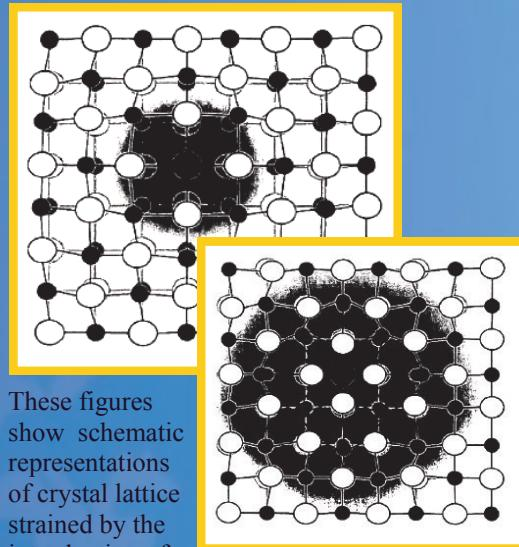
These figures show schematic representations of crystal lattice strained by the introduction of isovalent cation and aliovalent cation with ionic radii slightly larger than the host cations
