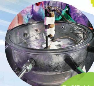
The BATLab is equipped with 4 mechanical abuse test systems to perform a variety of puncture, impact, or crush tests that can deliver up to
