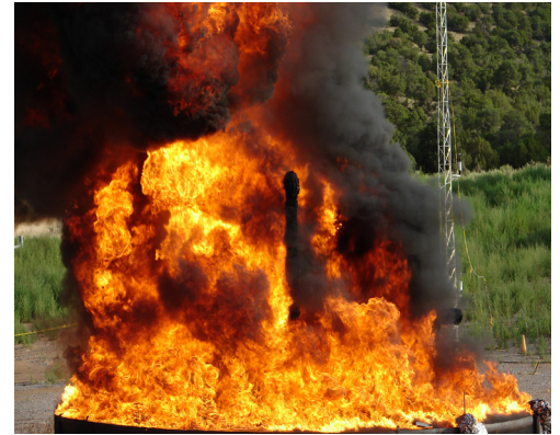
Full scale fire test of a spent fuel transportation container
