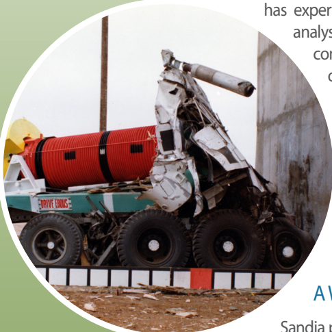
Crash test of a spent fuel truck cask
