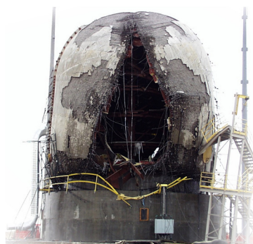
At 70-feet tall and 35-feet in diameter, this ¼ scale containment is the largest nuclear reactor containment vessel model ever tested to failure.
