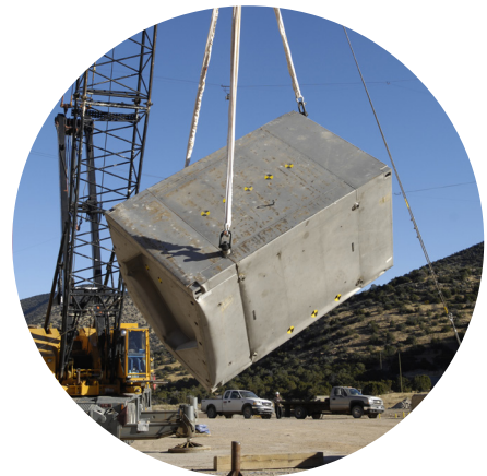
Puncture test of the Trupact-III transuranic waste transportation container
