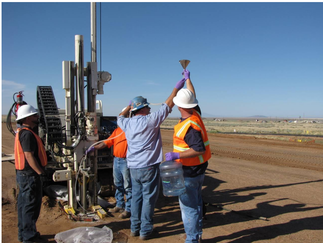
Figure 2-3 Hydrating the bentonite plug by pouring deionized water into tubing inserted into the Geoprobe rods at soil-vapor well MWL-SV01 location, August 7, 2009 (view to the southwest).
