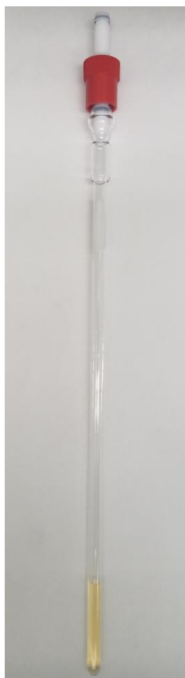
Figure 1. NMR experimental setup. (a) Picture of NMR tube with an PTFE/FEP insertion and (b) schematics of the NMR setup.
