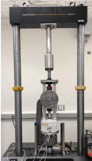
Figure.17 The MMR PTO with flywheel to increase equivalent mass
