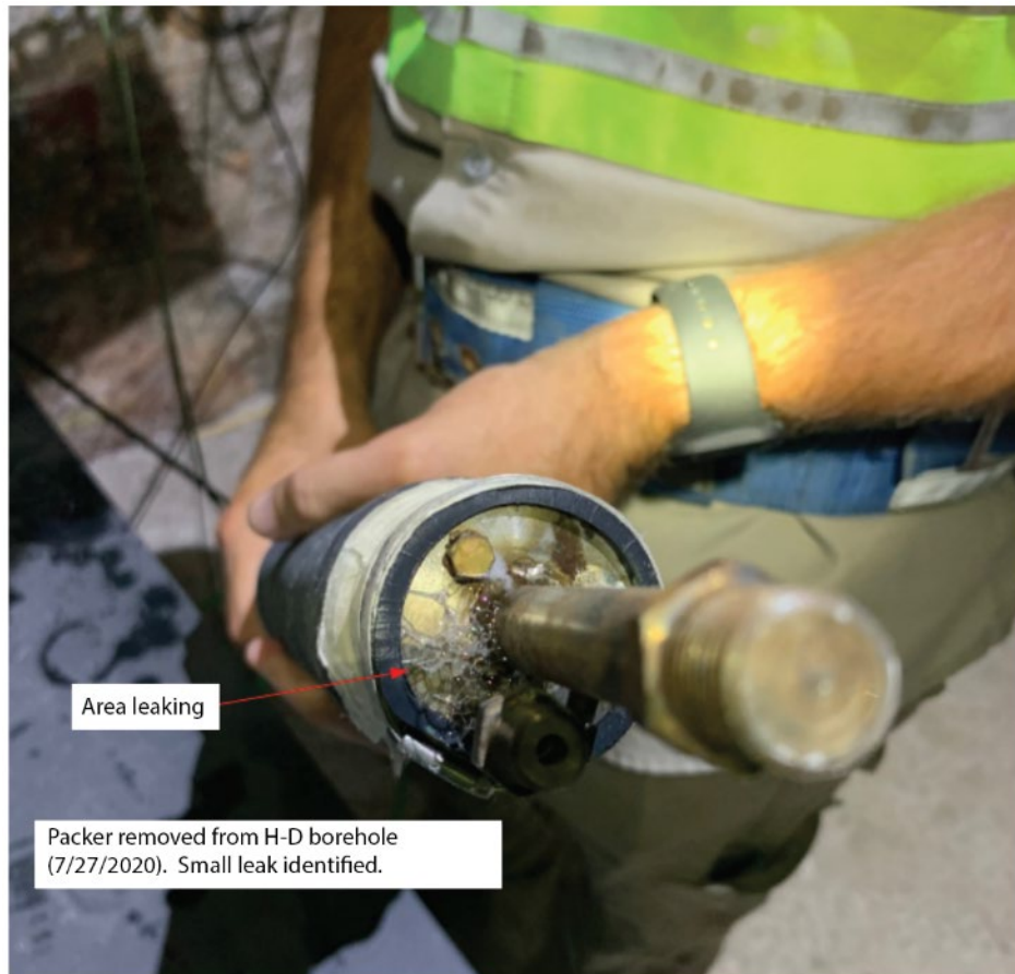
Figure 6-2. Leaky packer detected during permeability experiments.
