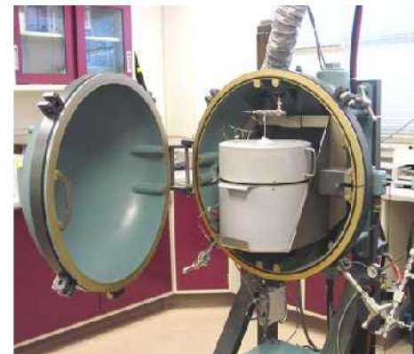
The SNL Accelerating Rate Calorimeter (ARC) is used to analyze thermal runaway in a variety of battery materials.
