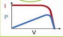
**6. DC and Mismatch Losses** – DC string and array IV curves are affected by wiring losses and mismatch between series connected modules and parallel strings.
