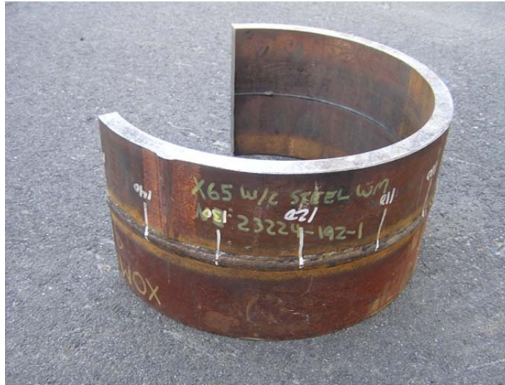
Figure 3. X65 steel girth weld supplied by ExxonMobil.
