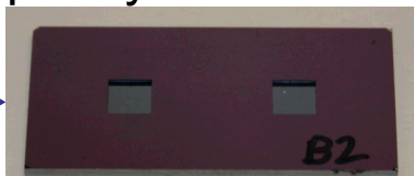
CSAM Large wafer bow, poorly bonded
