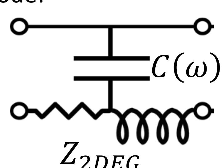
$$Z_0 = \sqrt{\frac{Z_{2\text{DEG}}}{i\omega C(\omega)}}$$
