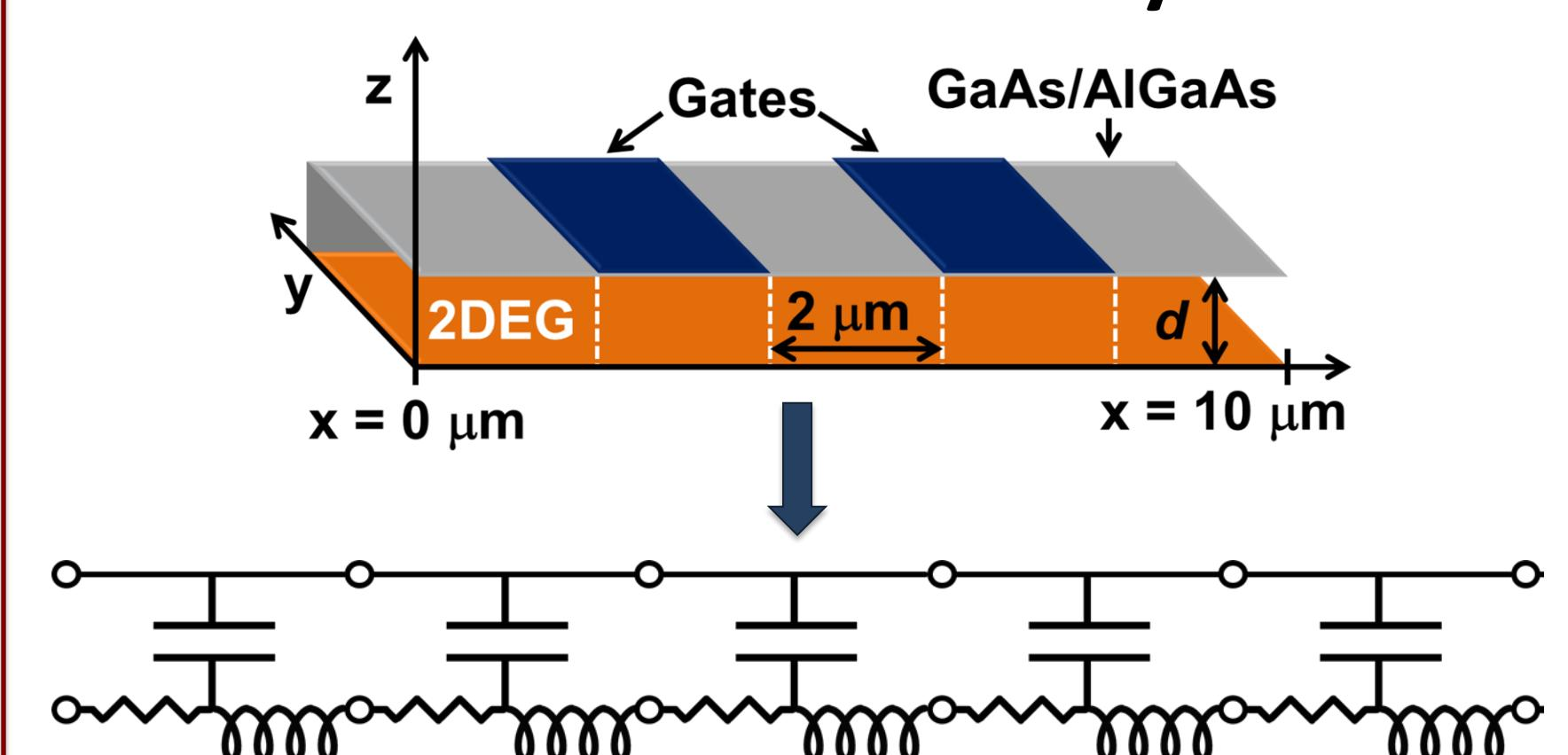
Solution for an inhomogeneous cavity with step-like boundaries between TL elements is reduced to matrix multiplication:
