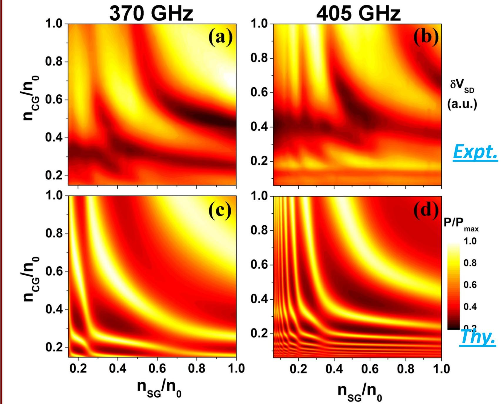
Experiment and model show transition from plasmonic spectrum of a homogeneous cavity to coherent interaction of independently tuned sub-cavities below SG & CG
