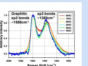
Characterization of carbon transition from sp<sup>3</sup> to conductive sp<sup>2</sup> as a function of temperature proved challenging due to heterogeneity of char formation.
