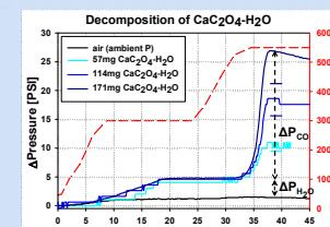
Comparison of model predictions and experimental measurements of gas yield pressurization for decomposition of ammonium carbamate (left figure) and calcium oxalate (right figure). Some deviations occur at higher carbon monoxide yields for calcium oxalate system.
