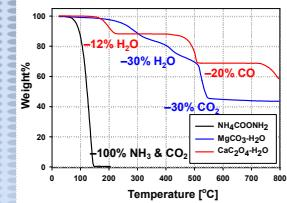
Gas yield per mass of inorganic reference materials was determined by TGA, converted to moles, and used with the ideal gas equation to calculate anticipated pressure increases in confined volumes.
