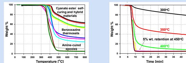
Weight retention depends greatly on the type of polymer (left figure). Isothermal TGA of an amine-cured epoxy material (right figure). Basic conductivity data (not shown) demonstrates that conductivity becomes an issue for residues when heated above 550-600°C.
