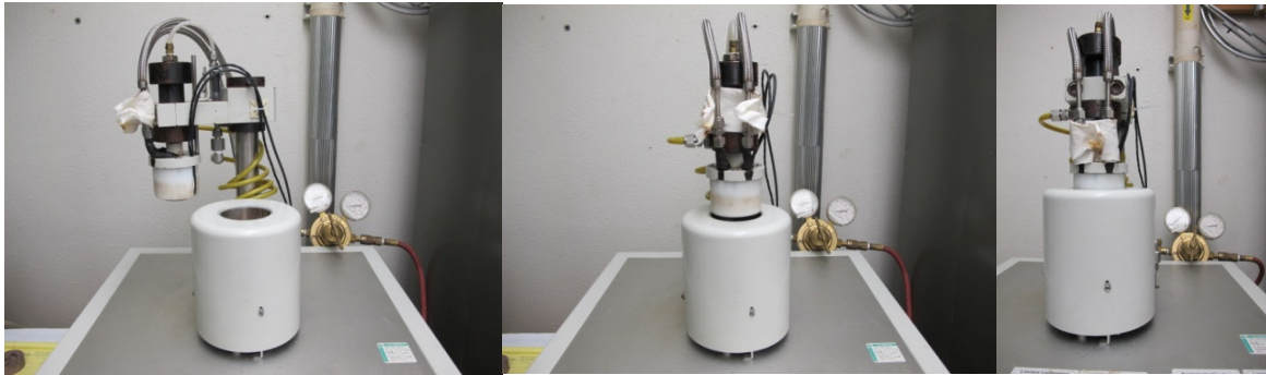
Figure 2: From left to right: The test stack in the opened position, ready to be loaded; the test stack with sample loaded, ready to be clamped; the test stack clamped by bottled nitrogen (out of sight) at 70 psi.
