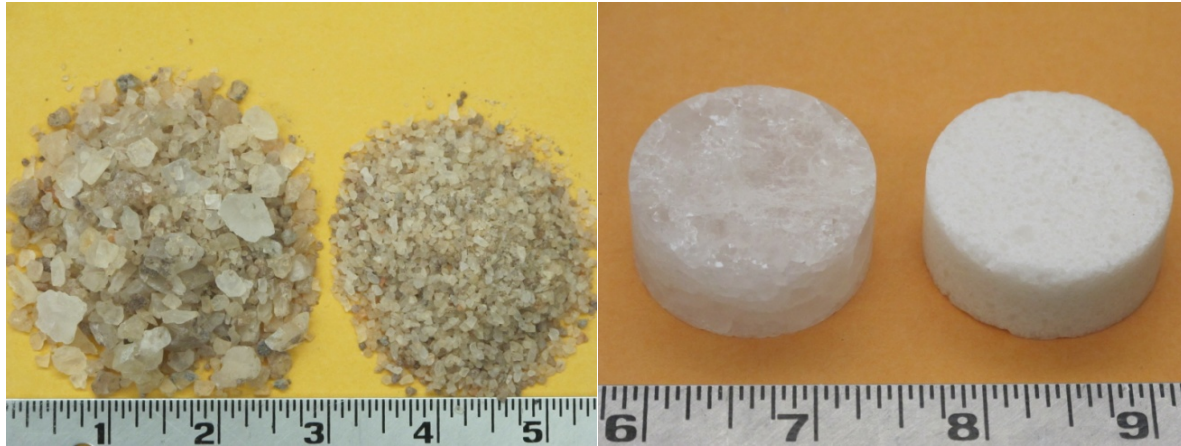
Figure 6: A) Non-sieved (left) and sieved (right) mine-run crushed salt used to make samples of variable porosity; B) domal salt (left) and salt lick salt (right) 38.1-mm cores used to obtain thermal conductivity measurements at low porosities. Scale in inches.
