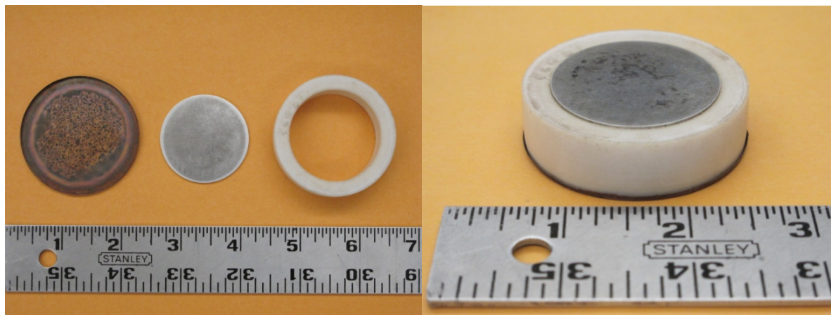
Figure 7: A) Components of the sample holder, from left to right: copper foil base, aluminum top cap, Teflon ring; B) the assembly ready for testing. Scale in inches.
