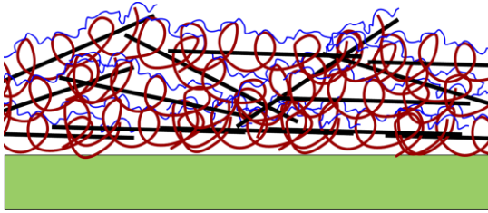
Figure 2.1. Pictorial representation of a layer-by-layer manufactured (\text{MWNT-PSS/PVA})_n thin film. PSS chains (helical red lines) wrapped around MWNTs (straight black lines) with deposited PVA (thin blue lines).
