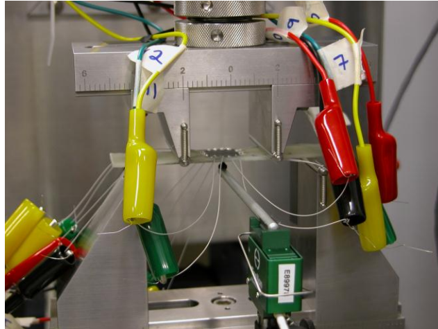
Figure 3.5. A 4-pt. bending specimen placed in the flexure fixture.
