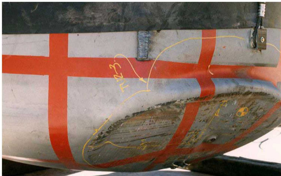
Figure 6-53. TRUPACT-II Test Unit CGOC Impact HAC Drop Test.
