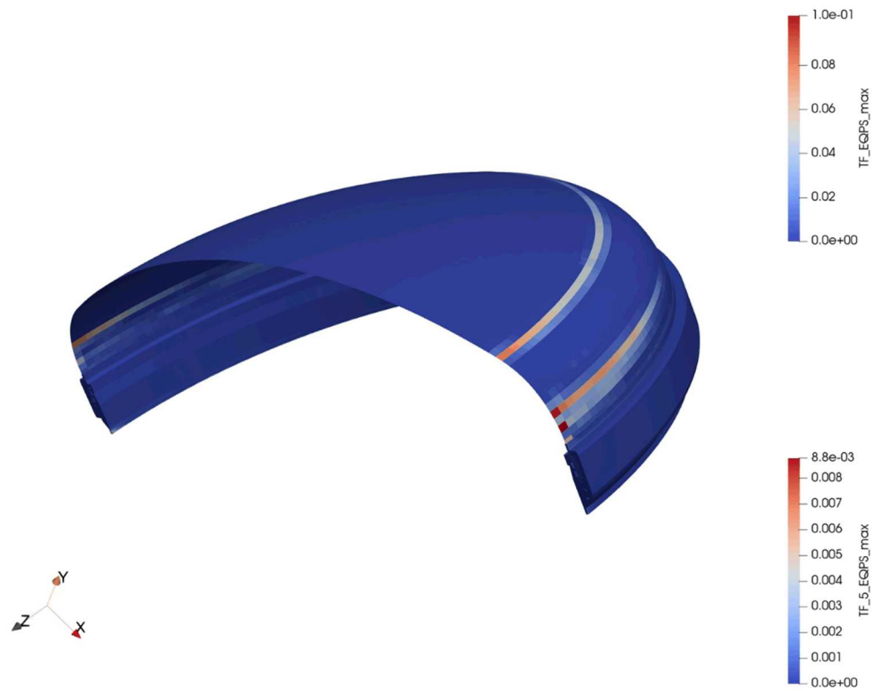
Figure B-16. CGOC Impact 30-mph [TF\epsilon^p]_{max} top shell and flange.
