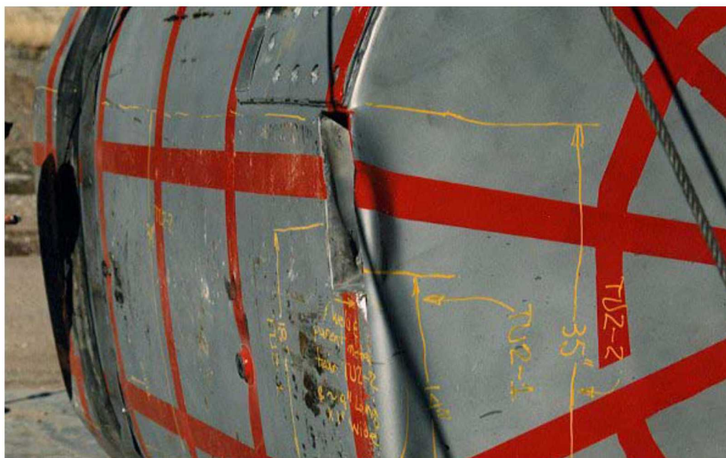
Figure 6-49. TRUPACT-II Test Unit Side Impact HAC Drop Test.
