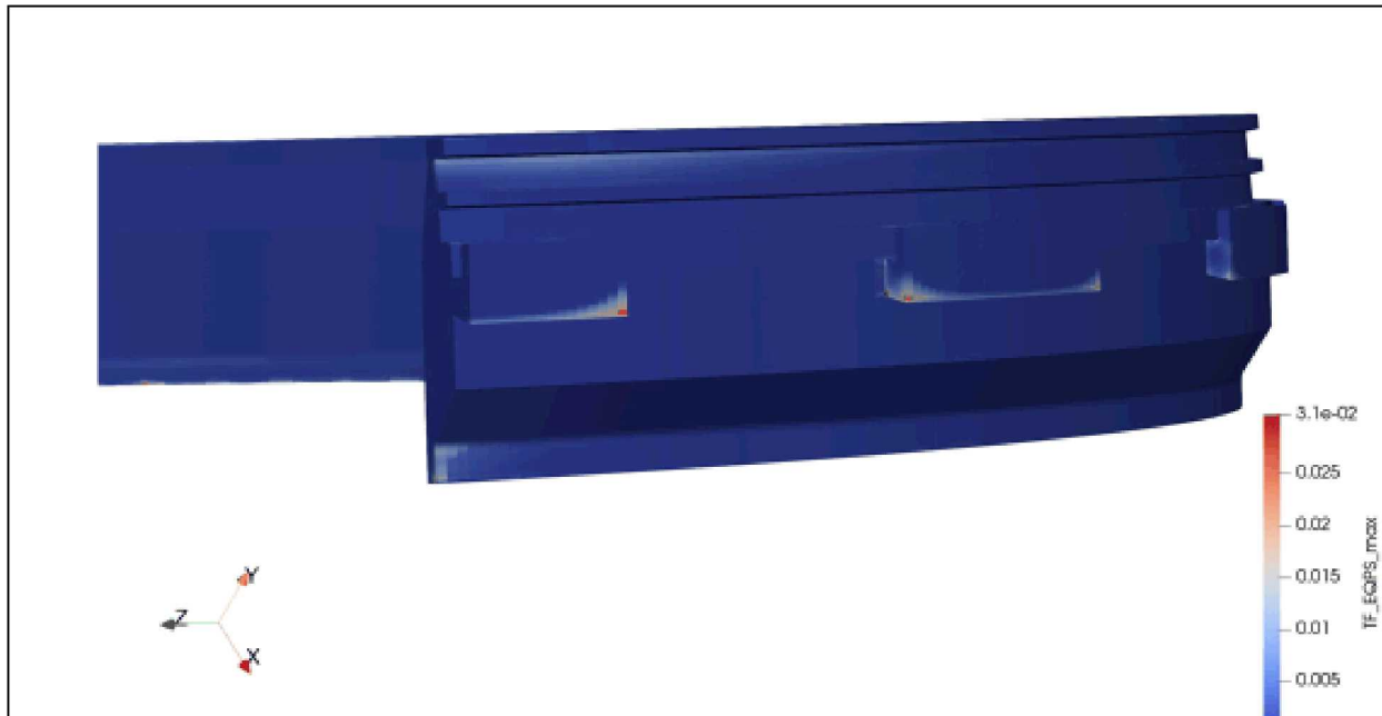
Figure B-18. CGOC Impact 30-mph [TF_{eq}^p]_{max} lower flange.
