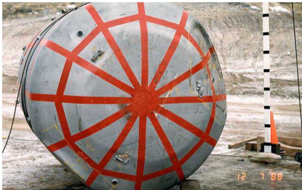
Figure 6-51. TRUPACT-II Test Unit Top Impact HAC Drop Test.
