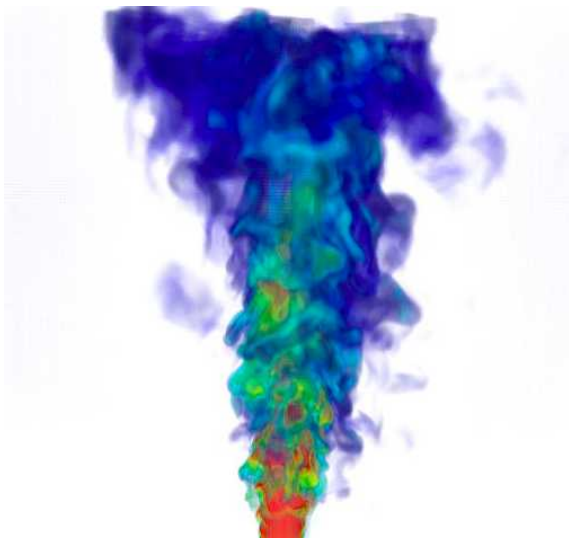
Figure 1: Volume rendering of a conserved scalar mixture fraction field in a turbulent open jet ( Re = 6,600 )
