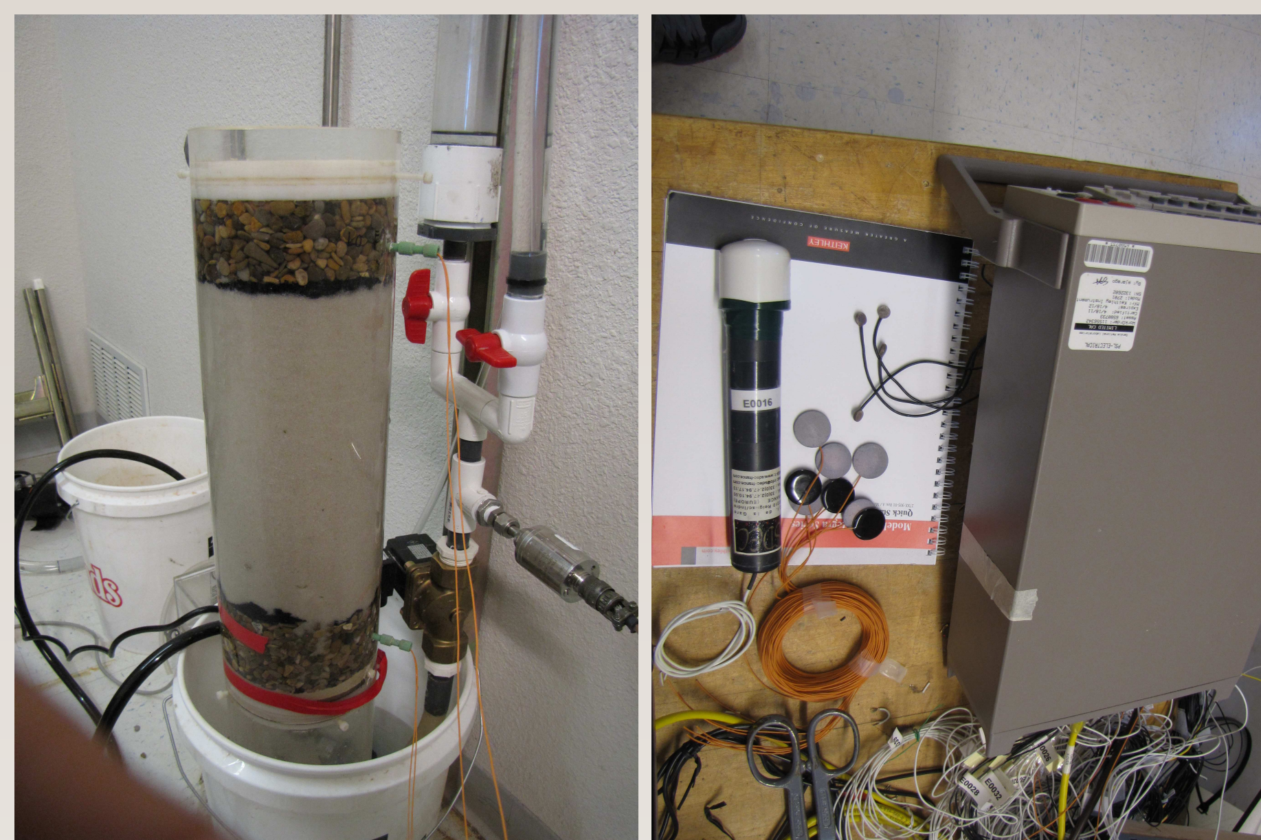
FIGURE 4: Falling-head permeameter and the electrodes used in the experiments. Permeameter SP data obtained with biomedical electrodes.
