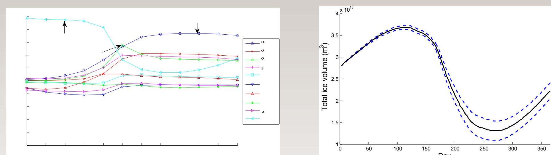
Standardized regression coefficients for a selection of ten parameters for Arctic ice volume (left) and the mean and 2-sigma variations of total ice volume for the single year run (right).
