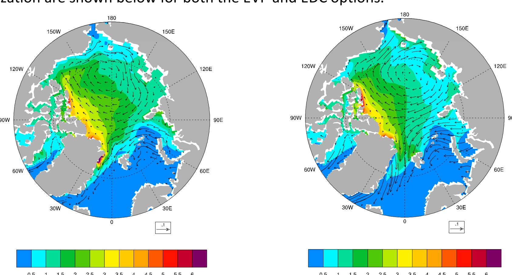
Ice thickness contours and velocity vectors after a single year run of CICE on a 1 degree grid with the EDC (left) and EVP (right) rheologies.
