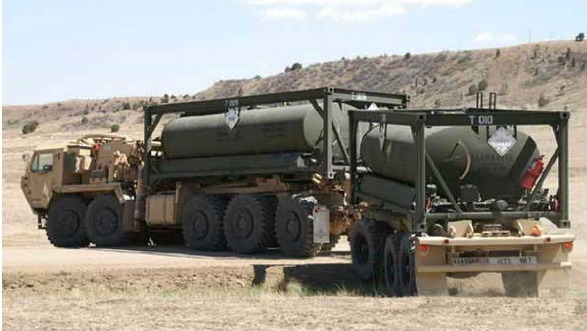
Figure 4. M1120 Load Handling System HEMTT with Trailer Transporting Two 2,500-Gallon MFS Tank Racks
