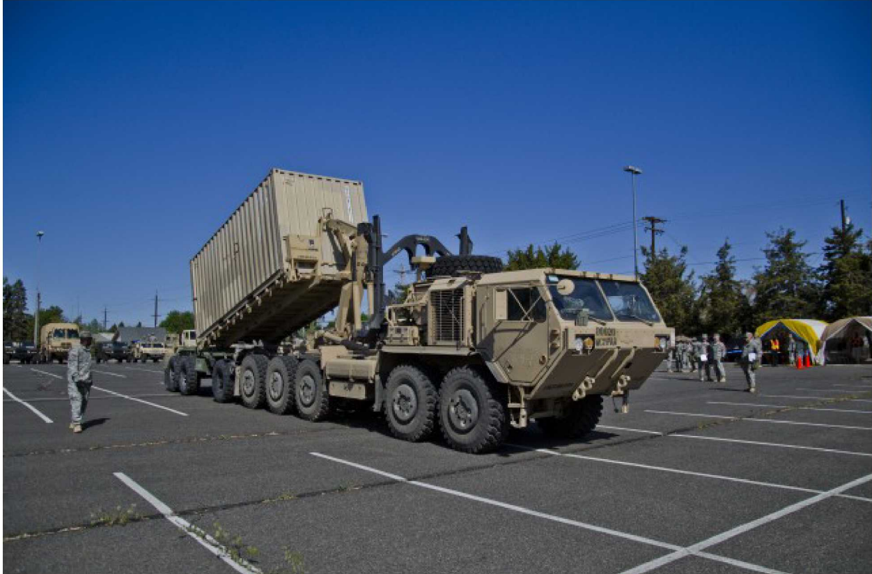
Figure 5. M1075A1 PLS unloading a 20-foot ISO Shipping Container
