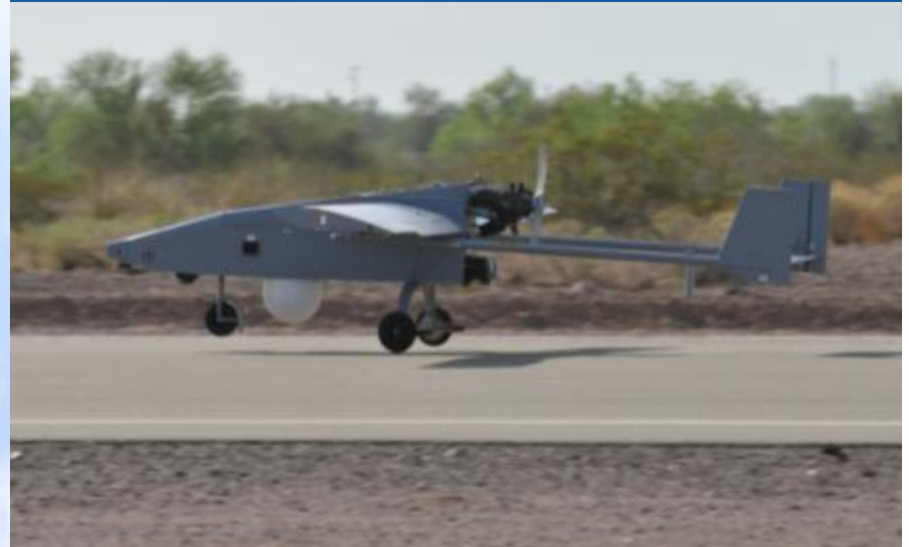
A Class III UAV outfitted with a Sandia-developed SAR.
