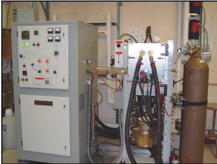
Ultra-high Temperature Furnace with Rapid Quenching Facility (up to 2400°C) (UW-Madison)
