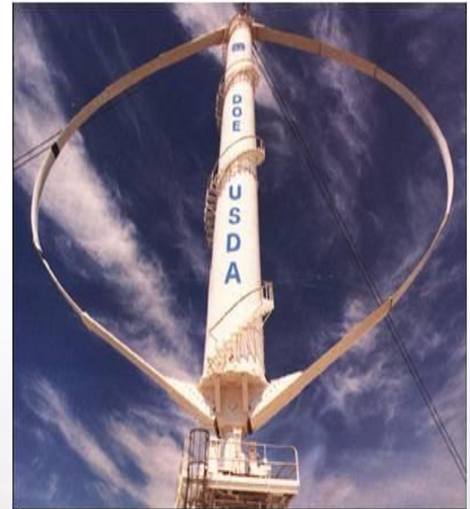
The DOE/Sandia 34 meter VAWT.
