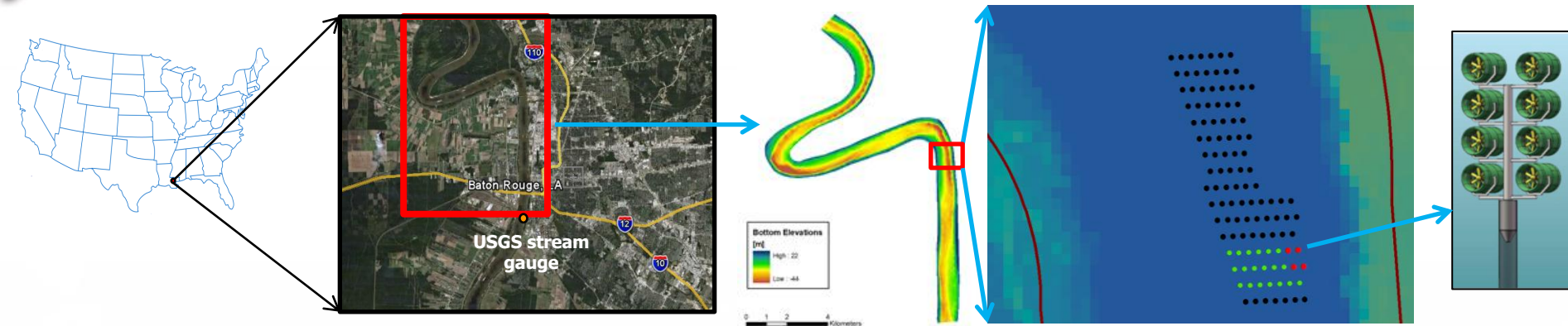
~ Hub height velocities with 23-pilings (112 MHK-turbines)
