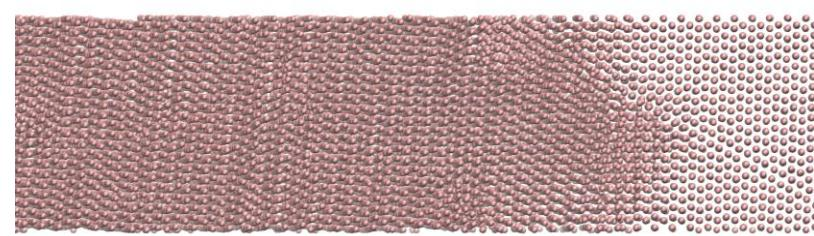
Examples of shock response of beryllium for three different shock piston velocities. At 3 km/s the material deforms elastically and plastically, at 5 km/s an amorphous solid is produced, at 8 km/s the material is fully melted.
