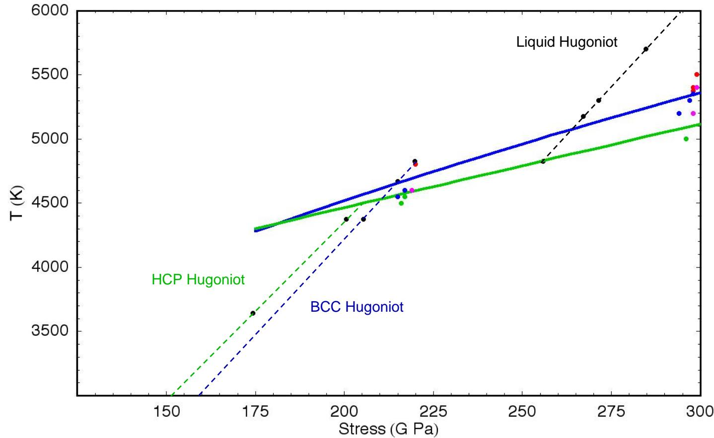
Our QMD calculations are consistent with the Z data and provide new insight into the Be phase diagram
