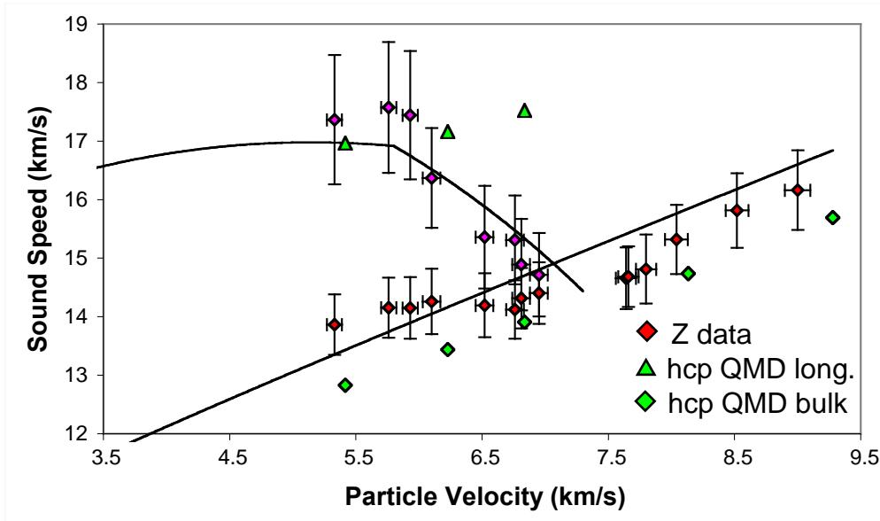
Ultra-high velocity flyer plate experiments on Sandia's Z machine, from Desjarlais, Knudson and Lemke, SCCM 2007
