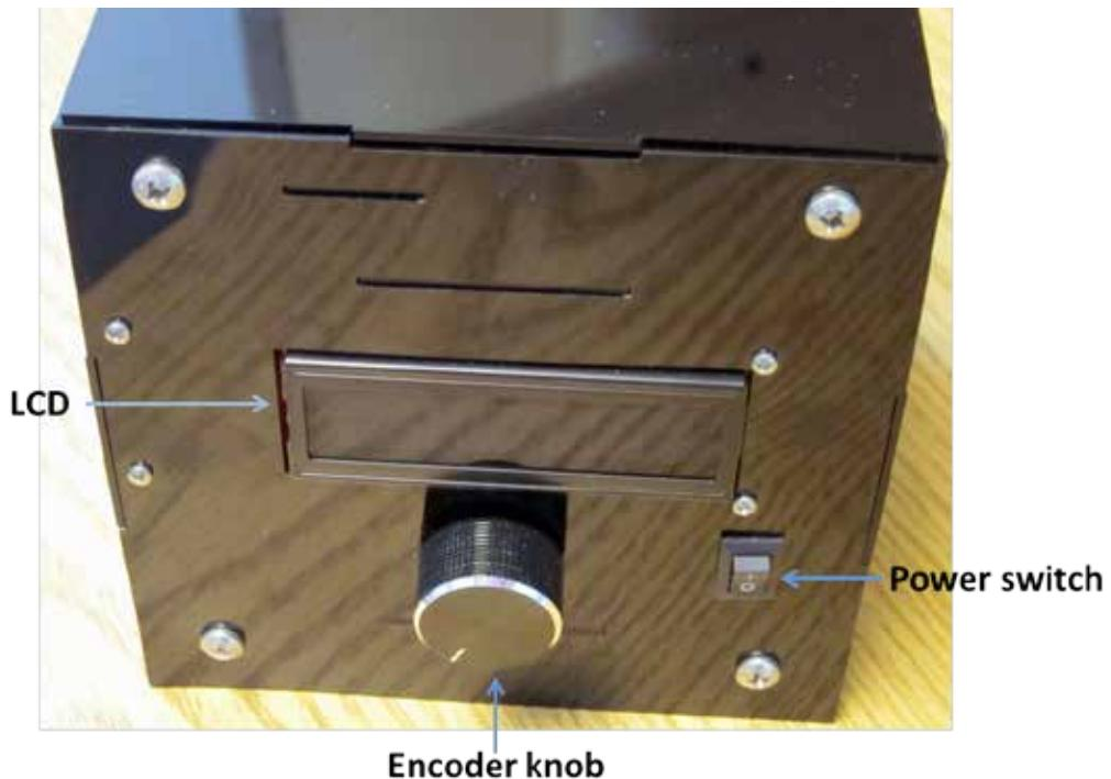
Front face of the demonstration prototype. The LCD screen displays instrument status. The power switch turns the instrument on/off. Rotate the encoder knob to switch between menu options. Depress the knob to select the displayed option.
