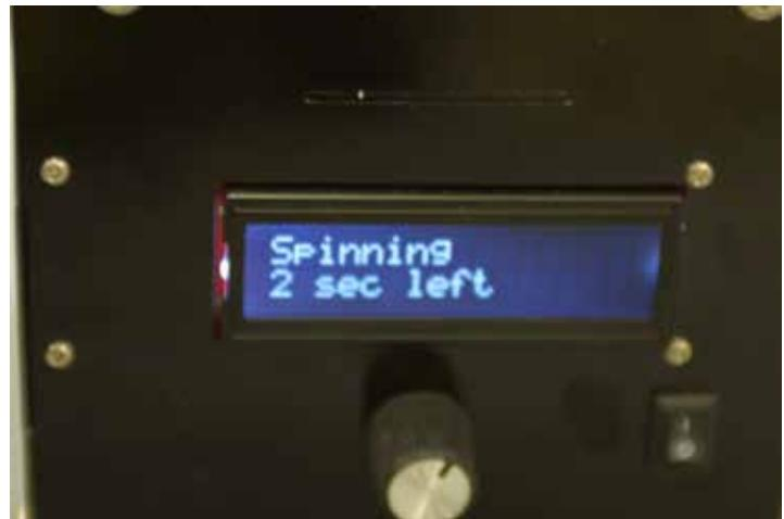
5. The LEDs will warm up and zero the instrument prior to analysis of the channels. The instrument will then step through each channel and read the fluorescence. The results are displayed on the LCD screen; scroll through the results by rotating the encoder knob.
