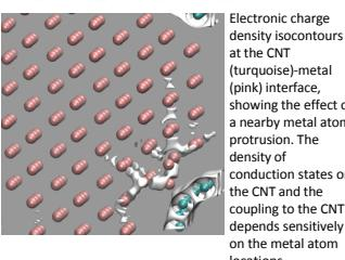
Phonon conductivity is correlated with structure and interface strength, much like the electronic conductivity. We investigate the structure-phonon transport relationship with idealized but realizable interface geometries.
