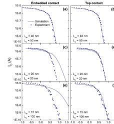
In order to fit the experimental contact resistance vs. contact length, we need a small value for the CNT-metal coupling strength.
