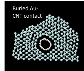
Post-Annealed Au-CNT contact, showing the formation of a dislocation in the metal due to the nanotube
