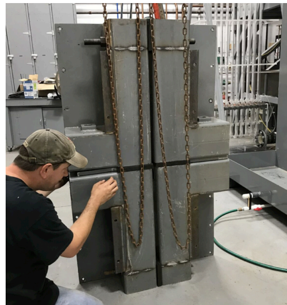
Figure 11: LPS full-scale seal test rig, in preparation for leakage test.
