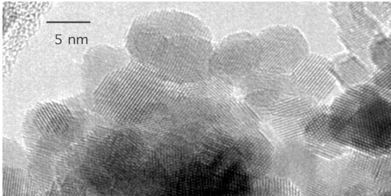
**Figure 2.** TEM micrograph of a hydrothermally derived Gd-doped ceria powder.
