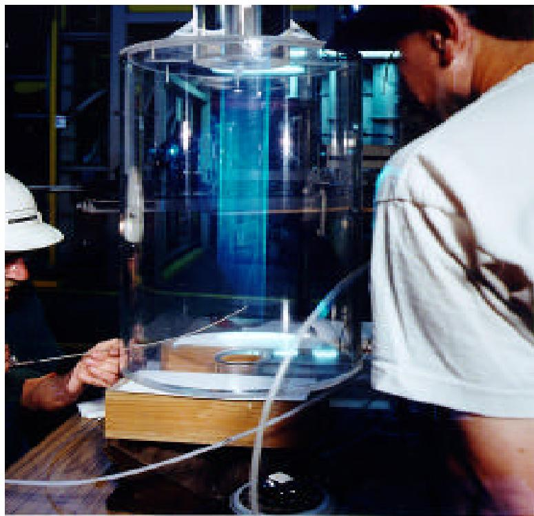
*Figure 10. Cold flow visualization studies used to verify numerical modeling results*
