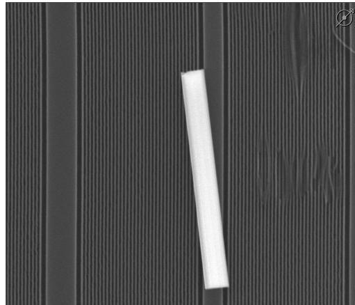
The wire is then rotated to minimize optical feedback.
