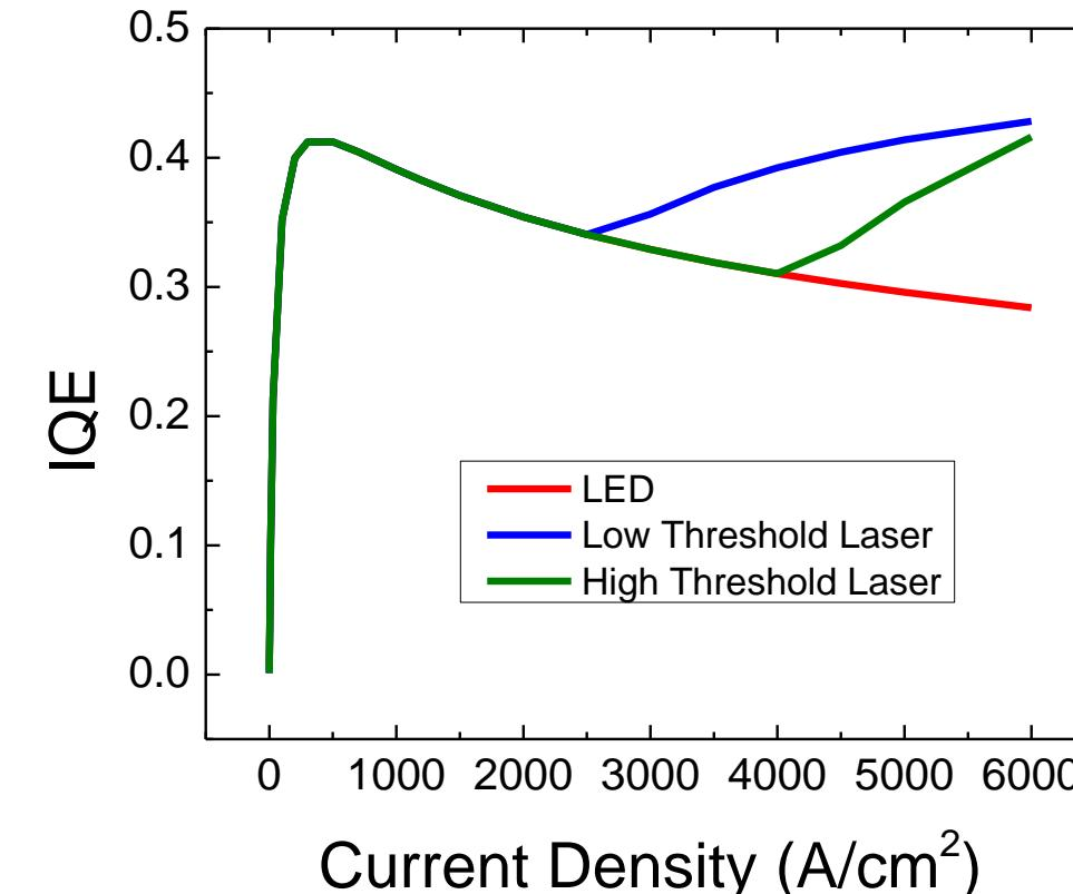
In a device with feedback the onset of stimulated emission overcomes the efficiency droop of the LED. Having a lower threshold means the droop is minimized at lower current densities.
