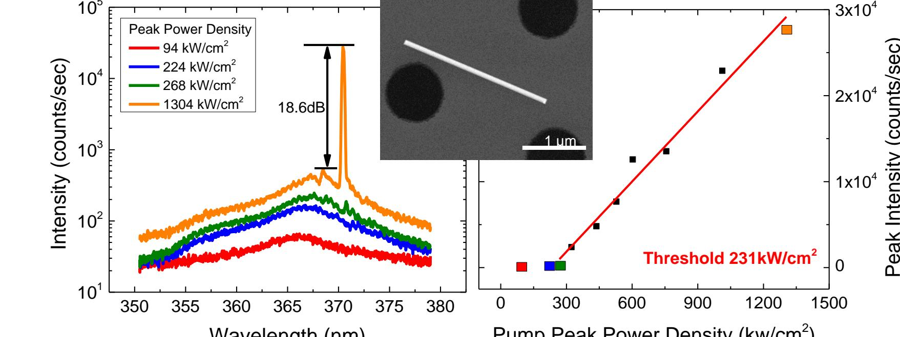
By reducing the width of the wire the number of competing modes is reduced. A 130nm x 5μm wire exhibits single mode lasing with a reduced threshold and high side mode suppression.
