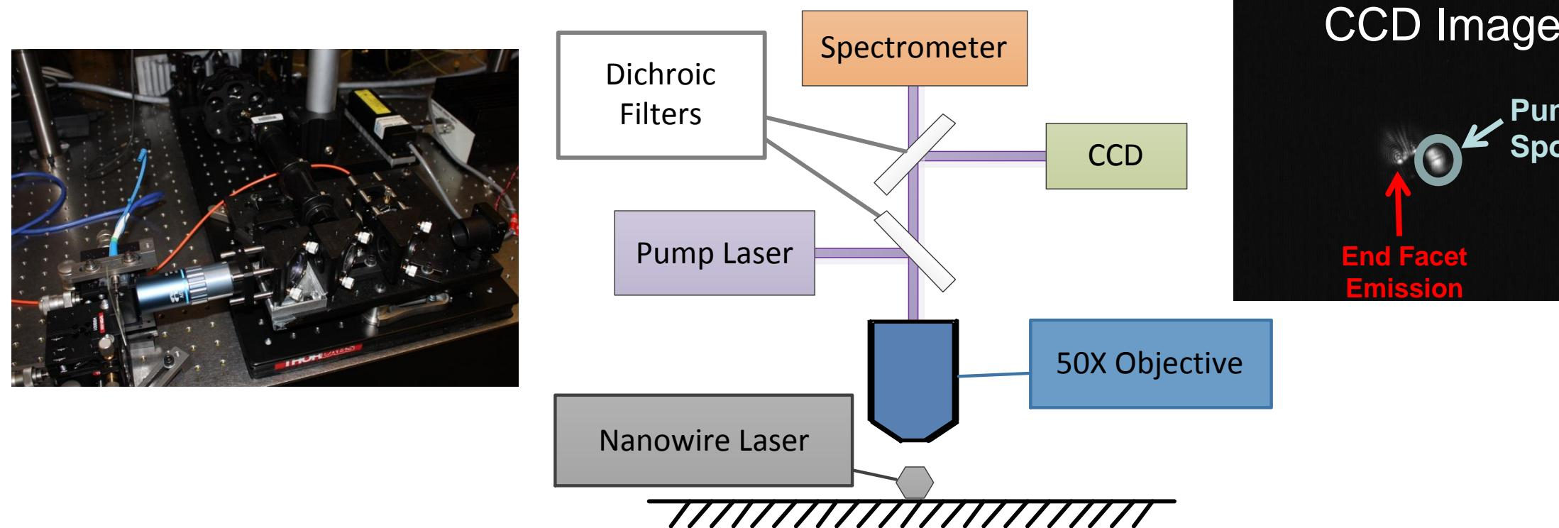
GaN nanowires lying on a substrate are optically excited through a 50x objective by a 266nm laser whose power is trimmed by a series of neutral density filters. Emission from the nanowire is collected through the same objective and is characterized by a spectrometer.
