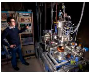
The Angle Resolved Ion Energy Spectrometer (ARIES) at Sandia/CA is one of the only instruments in the world that has been specifically optimized for investigating hydrogen on surfaces.
