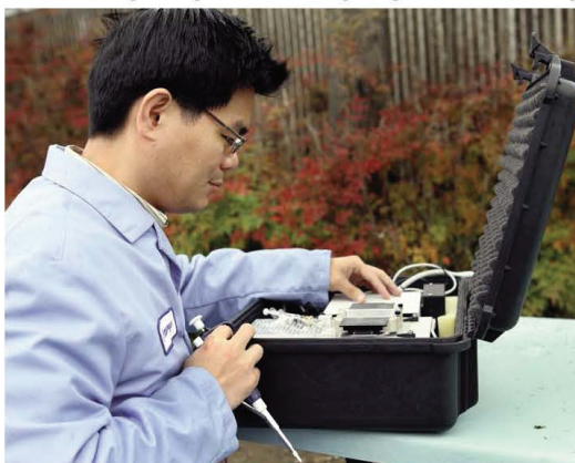
HANYOUNG KIM (8621) checks out the Rapid Threat Organism Recognition (RapTOR) device prototype. The digital microfluidic hub, visible inside the case, serves as the "Grand Central Station" of the device, routing and managing samples for speedy identification and characterization.
