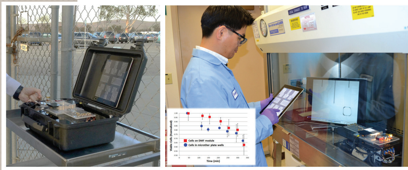
Figure 12: (Left) Sandia DMF Hub-based system packaged for deployment in the field. (Right) DMF Hub for automated cell culture processing in a biosafety containment hood. The embedded graph shows the high cell viability cultured on the DMF hub. The remote operation through a handheld GUI interface provides safe but real-time experimental control of potentially infectious or hazardous samples.
