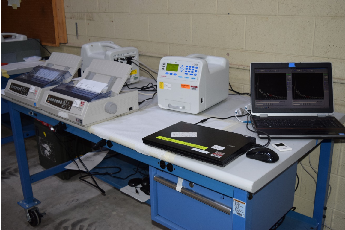
iSolo counters with printers for recording beta counts and laptop for an electronic save of count data. Laptop on the right is for the NaI-URSA.
