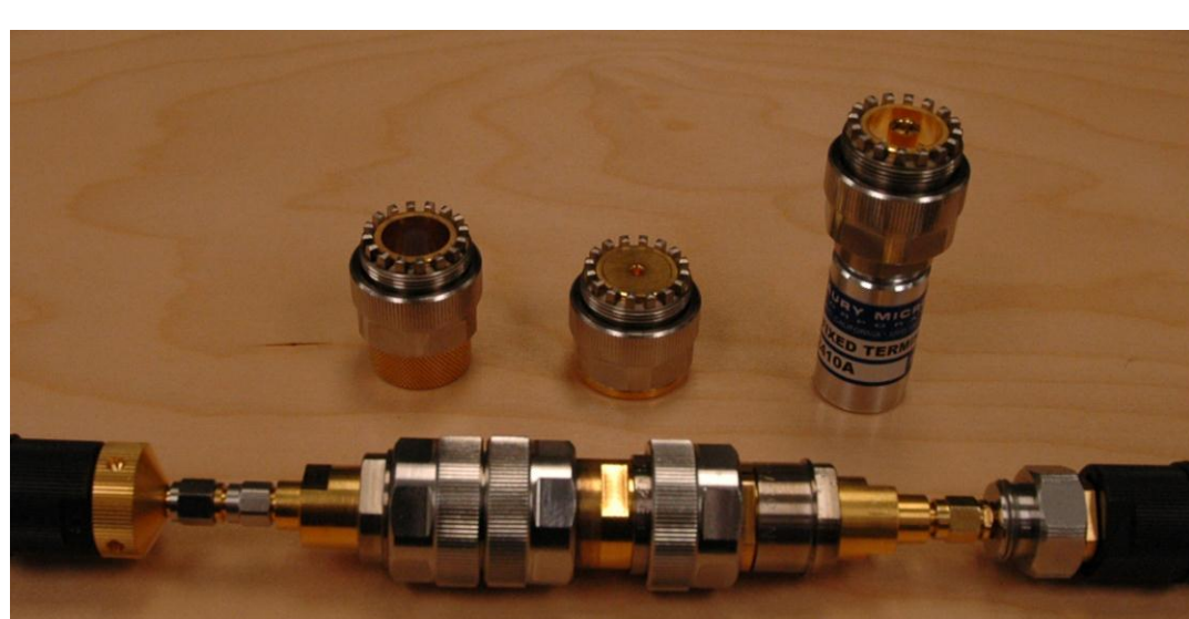
Coaxial test fixture for characterizing RF properties of blade materials and RAM
