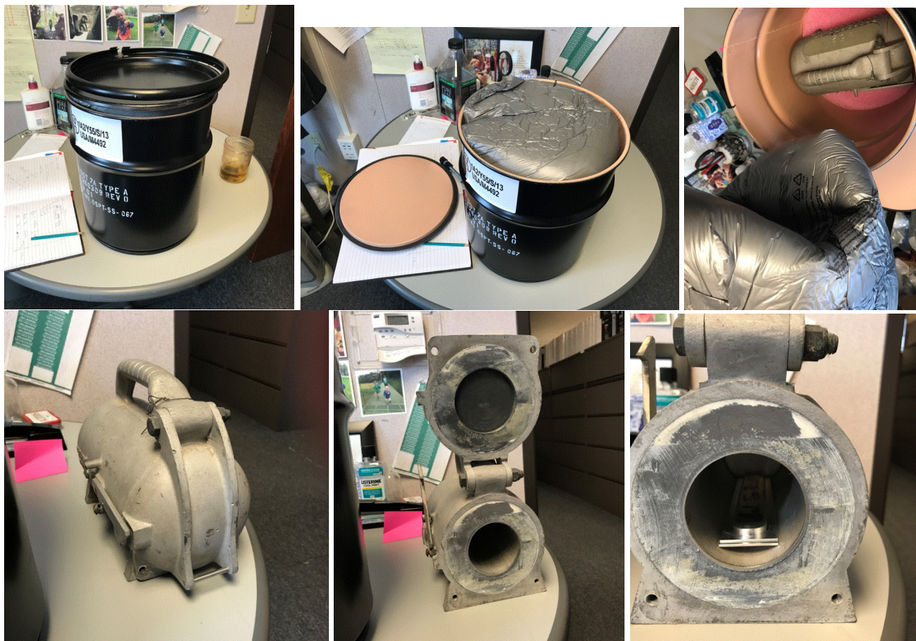
Figure 1: Pictures of a certified shipping system to be used for shipments of irradiated bismuth targets from UW to LANL. The heavy B52 pig was not required for shielding, but it will be used as it was provided at no cost to the studies.
