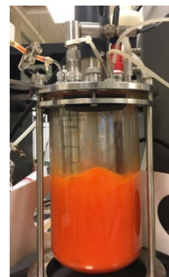
742 743 Fig. 6 Xylose fed-batch fermentation of the SR8B strain using Verduyn medium. The bioreactor 744 picture on the right was taken at 80 h. 745
